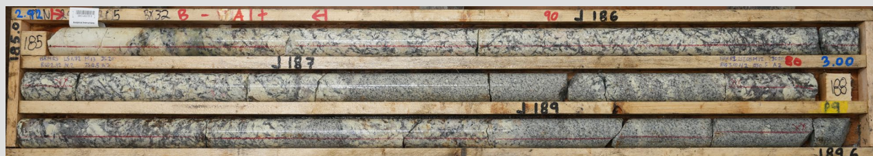
PLN25-205: Strong bleaching in top of basement below UC
